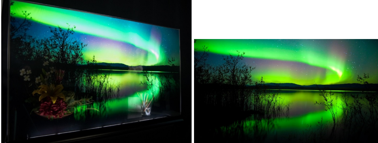
Figure 3 - Full screen image on a Planar LookThru OLED transparent display. To the right is the image as it appears in Photoshop (note the black is opaque in the image). Note: there is a light strip in this image that is not part of the product.
