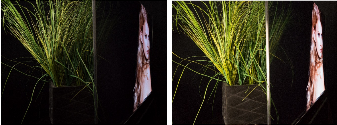
Figure 7 - Minimal lighting behind a display renders the display more opaque. Bright lighting behind the display makes the screen appear more transparent, as evidence by the grass behind visible through the display in the second image when it is not visible in the first image.
